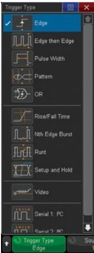
Figure 41. Wide array of advanced parametric trigger modes.
