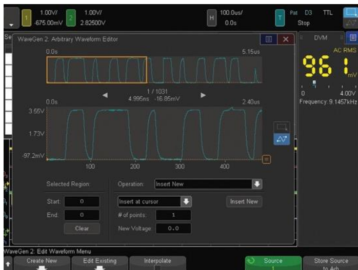
Figure 23. WaveGen arbitrary waveform editing screen.
