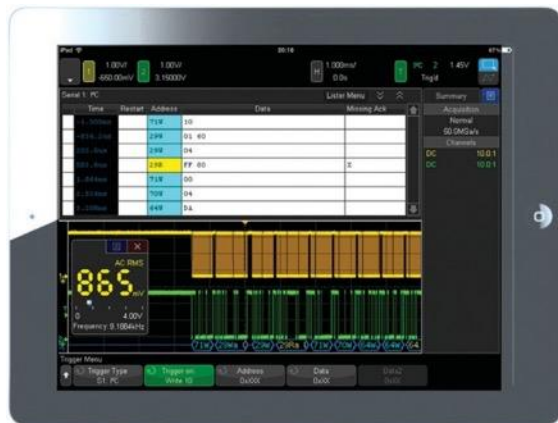
Figure 37. Tablet virtual front panel control.
