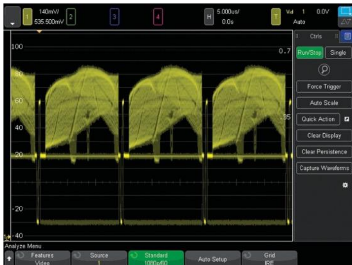
Figure 27. Triggering on 1080p HDTV signal analysis.
