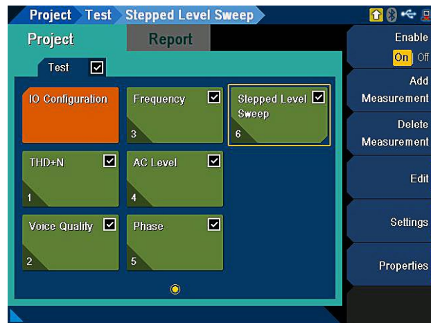
Figure 10. The test sequence control function comes with a selection of pre-configured measurements. It allows users to select the most frequently used test sequences for their daily measurement.
