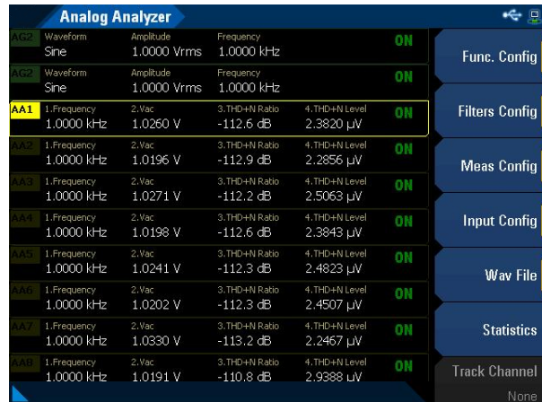
Figure 5. The U8903B's GUI, showing 8 analyzer channel measurements.
