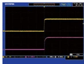
The CC Priority Feature Effectively Limits the Occurrence of Inrush Current and Surge Voltage when the Supplied Voltage Rises to the LED Forward Voltage
