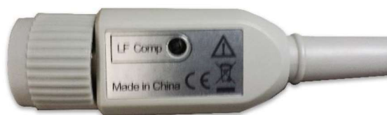
Figure 2. Low-frequency compensation adjustment (for N2840A/41A/42A/43A/53A)
